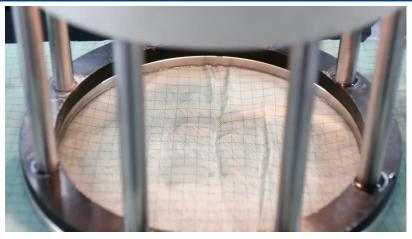
**Resistance to water penetration** measures the water pressure the fabric can withstand before leakage occurs.
