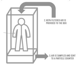
Limitation: due to the high variation in particle generation between individuals, one can only compare relative performance of garment systems if the test person and the test parameters are identical
