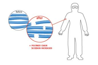
Impact of gamma radiation exposure seen in reduction in tear strength with increased nominal received dose
