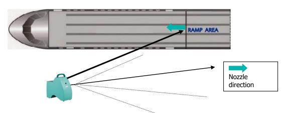
F. <u>For the cargo holds</u> Position the DAF-3000 as near as possible to the door and direct the nozzle towards the bottom of the hold.
