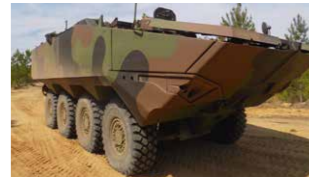
The full armour package for SAIC's ACV 1.1, including applique armour, spall liners and lightweight composite floatation boxes.
