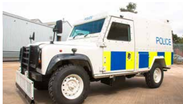
Designed, integrated and armoured composite Snatch Land Rovers for military and law enforcement operations.
